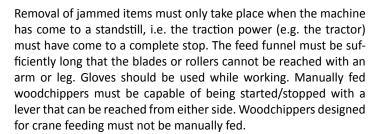
Woodchippers often reach noise levels above 80 dB(A). Hearing protection must be used when working with machines emitting noise above 80 dB(A). Noise emitted from the machines should be reduced where possible. When purchasing new woodchippers, seek out the quietest machines on the market.
